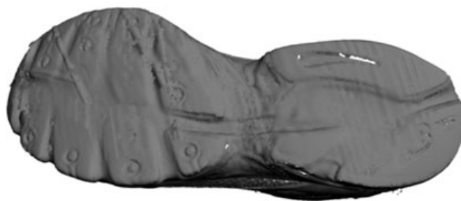
FIG. 3—A 3-D laser scanner image of the suspect shoe. Manipulation of the images in Figs 2 and 3 with an imaging software permits direct comparison and provides a demonstration tool for court purposes.
